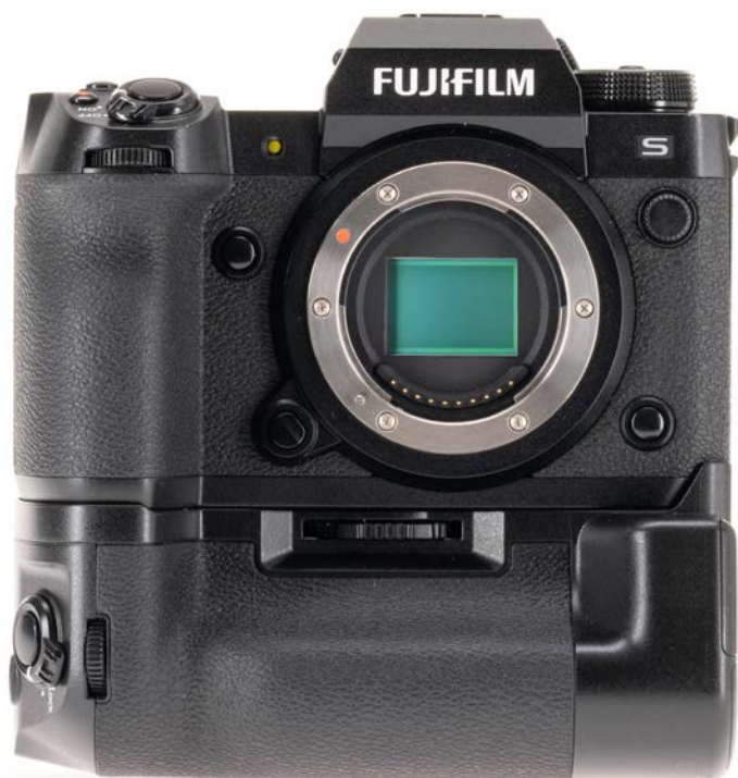
Fujifilm X-H2S with native X Mount (17.7 mm Flange Focal Depth)
