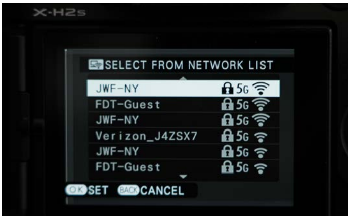
10, 11. Select Wi-Fi access point. If you have a mesh network, it's trial and error until you find the right node. Enter your Wi-Fi password. SET to enter.
