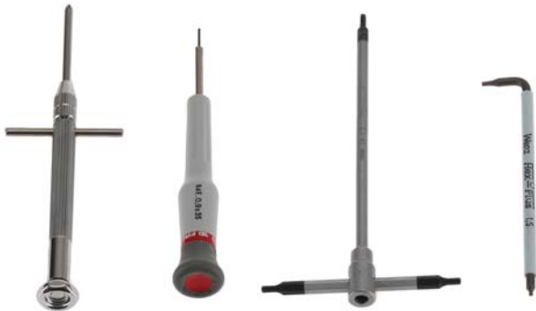
3. These are the tools you need: Small Phillips, 0.9mm hex, 2mm hex, and 1.5mm hex. It takes about 10 minutes to switch between formats.
