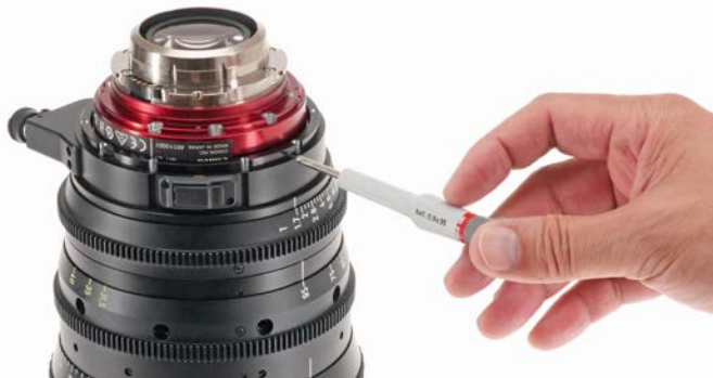
5. Loosen (but do not remove) 4x 0.9mm hex screws that adjust optical axis centering.
