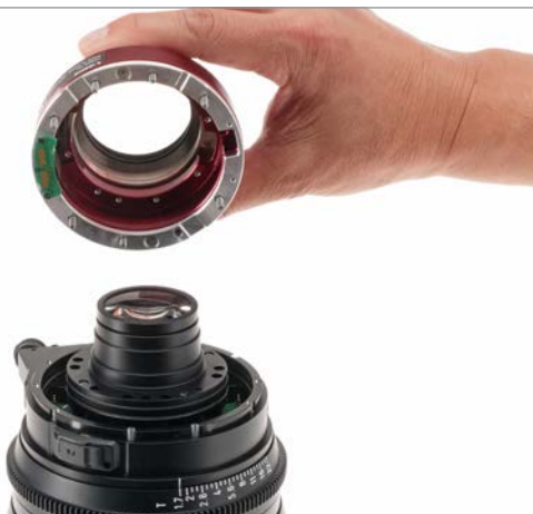
5. Loosen (but do not remove) 4x 0.9mm hex screws that adjust optical axis centering.
