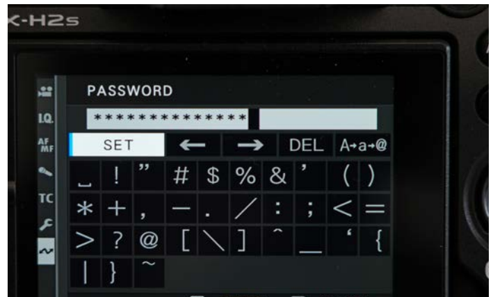
10, 11. Select Wi-Fi access point. If you have a mesh network, it's trial and error until you find the right node. Enter your Wi-Fi password. SET to enter.
