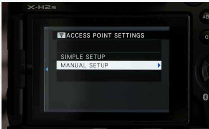
8. Select MANUAL SETUP. (SIMPLE SETUP is not as simple.)
