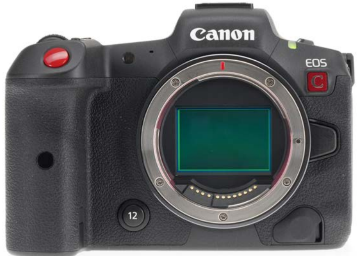
Shutter opens to reveal sensor when the EOS R5 C is turned on.
