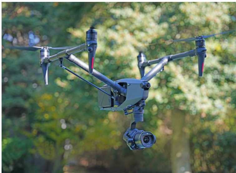
With rotors up in normal flight position, you can pan the camera 360 degrees without seeing the rotors.
