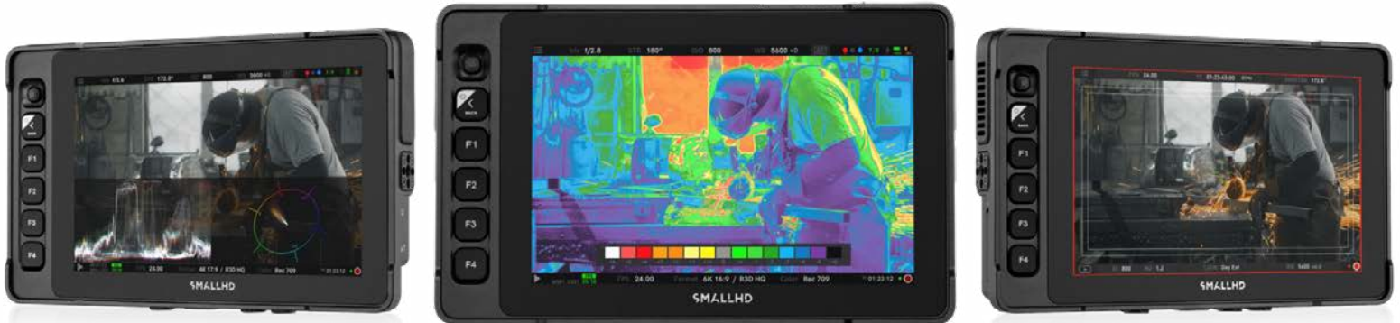
Ultra 7 has all the familiar PageOS pages, overlays and tools—including EL Zone “exposure meter.”
