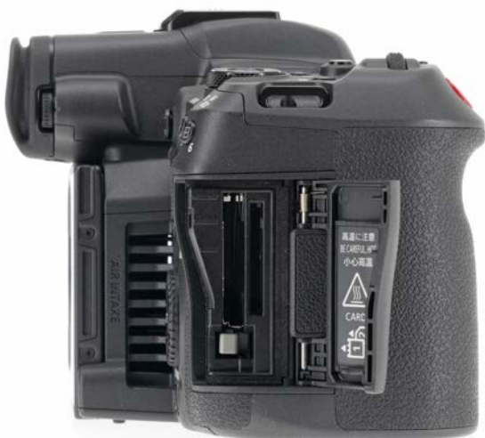
Camera right side with one CFexpress and one SD UHS-II slot
