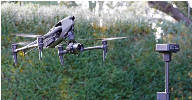
Inspire 3 flying with landing gear down lets you tilt the camera up 80 degrees without seeing the rotors. DJI D-RTK2 Mobile Station at right.
