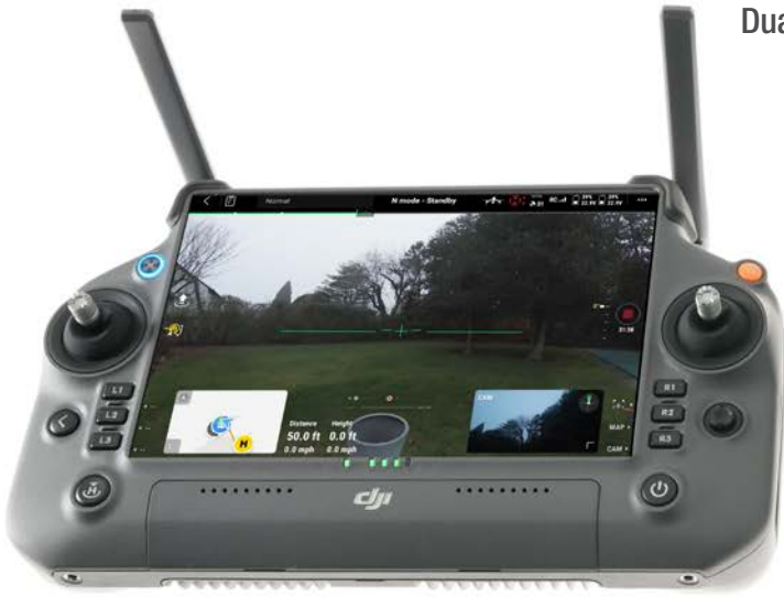
Pilot's Controller with FPV view displayed full screen and CAMERA view in window at lower right. Waypoints displayed in window at lower left.
