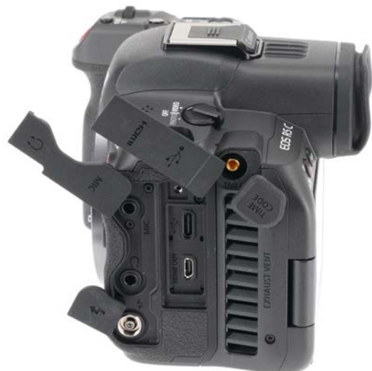
Camera left side ports: HDMI Out, USB-C, Timecode, Mic, Headphones
